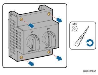
**Step 2** Remove the faulty PID switch.
