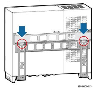
**Step 2** Remove the security torx wrench bound to the cabinet base and use the wrench to tighten security torx screws.
