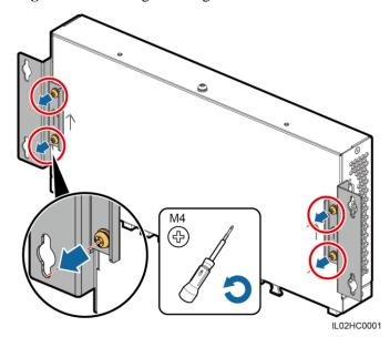
Figure 7-9 Removing mounting ears
