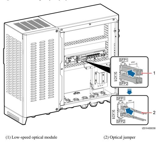
Figure 5-7 Connecting an optical jumper
