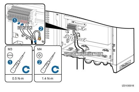
Figure 5-22 Connecting RS485 communications cables
