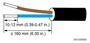
**Step 2** Connect the cable to the single-phase input switch.
