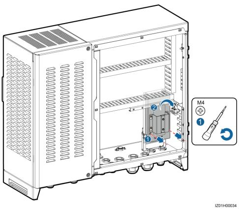
**Step 2** Remove the optical cable fastener.
