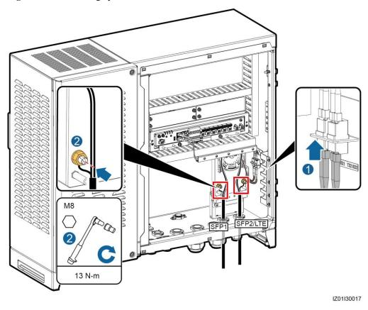
Figure 5-11 Connecting optical cables
