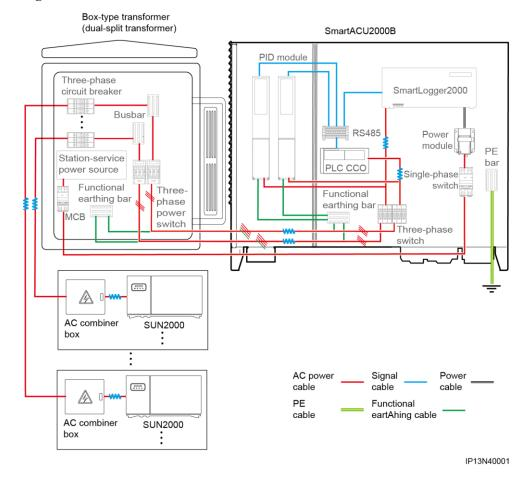
Figure 2-14 PLC communication mode
