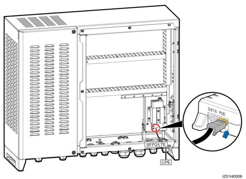
Figure 5-16 Connecting the CPE network cable
