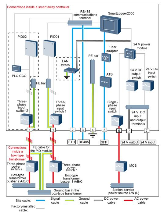
**Figure 2-16** Component connections (for the smart array controller supporting 24 V DC input and output)
