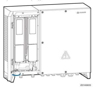
Step 2 Open the PID module maintenance compartment door, and remove the connection box cover.
