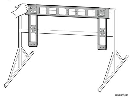
Figure 4-7 Determining hole positions
