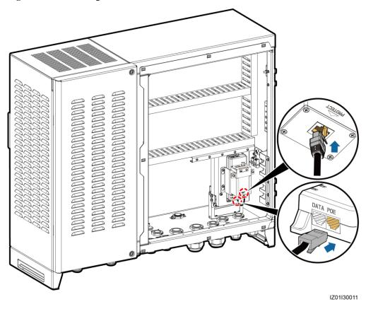
Figure 5-12 Connecting a POE module to a POE SPD
