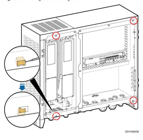
Figure 6-3 Removing reserved floating nuts
