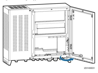
Figure 4-15 Using a support bar to stabilize a door
