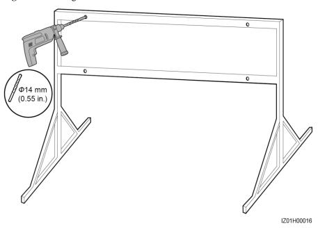
**Step 3** Align the mounting bracket holes with the drilled holes, insert M12x60 bolt assemblies (each being an expansion bolt with only a flat washer and a spring washer) into the holes through the mounting bracket, and secure them using the shipped stainless steel nuts and flat washers.
