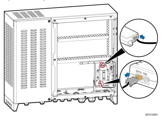
Figure 5-15 Connecting the POE module cable
