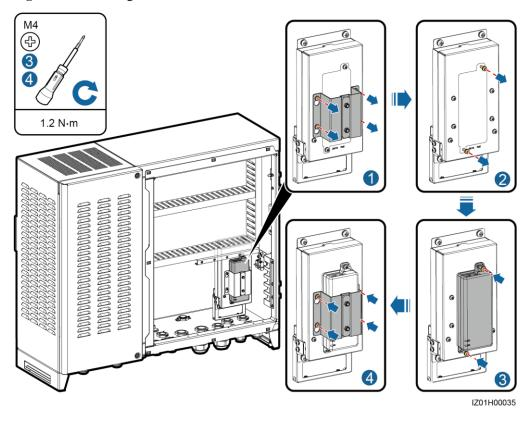
Figure 4-16 Installing a POE module
