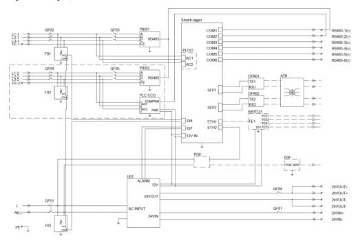
**Figure 2-12** Electrical conceptual diagram (for the smart array controller supporting 24 V DC input and output)
