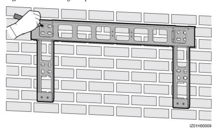
Figure 4-3 Determining hole positions
