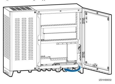
**Step 2** Close the main cabinet door and tighten the screws.
