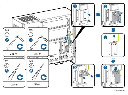
Figure 4-17 Installing a POE SPD
