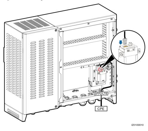
Figure 5-14 Connecting the CPE network cable
