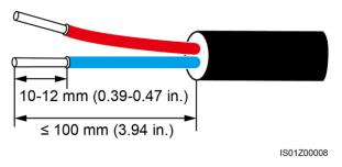
**Step 2** Connect the 24 V DC input power cable to the JX02 terminal block.
