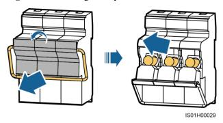
**Step 3** Install the new fuse and close the knife fuse switch box.
