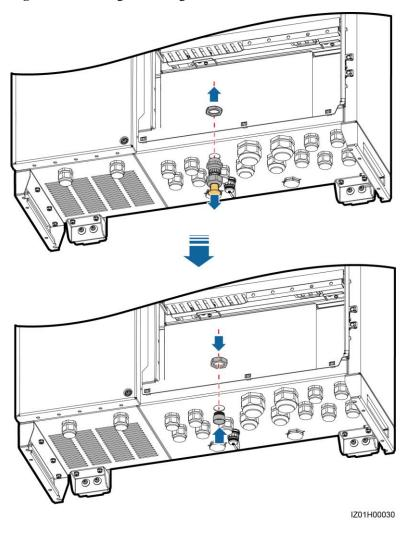
Figure 5-4 Installing tube fitting
