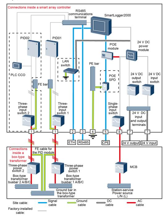
**Figure 2-18** Component connections (for the smart array controller supporting 24 V DC input or output)
