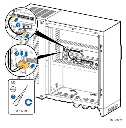
Figure 5-23 Connecting LAN switch cables
