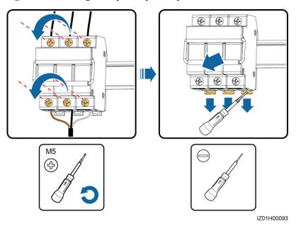
Figure 7-4 Removing a faulty three-phase input switch
