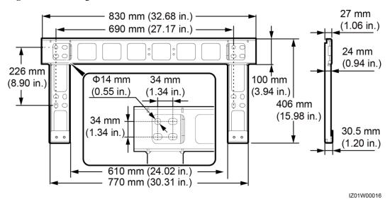
Figure 4-2 Mounting bracket dimensions
