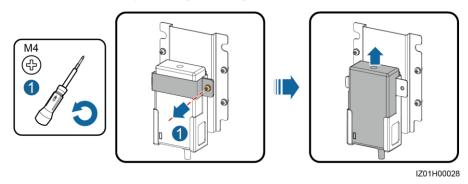
**Step 4** Install the new power adapter.
