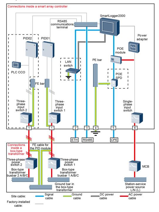
**Figure 2-17** Component connections (for the smart array controller not supporting 24 V DC input or output)
