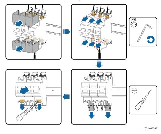
Figure 7-3 Removing a faulty three-phase input switch
